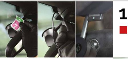
Use the included cleaning kit to degrease the windshield thoroughly. Position and stick the Pals sensor as high as possible with its cable up and behind the roof's part.
